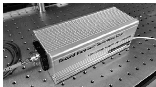
Fig. 6 Second harmonic generation unit with 460\ \sim\ 550\ \text{nm} tuning range.
